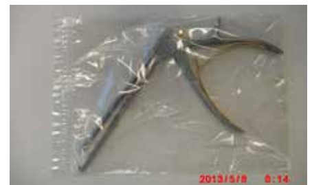
Fig. 6: Complete elution of a dismantlable punch into a PE bag
