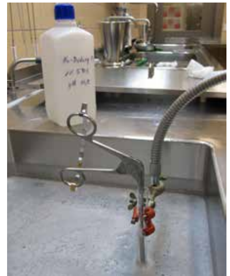
Fig. 5: Partial elution into a test tube of an instrument functional end, using ultrasound additionally
