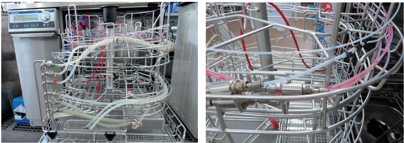
Image 1: AER with connected 2000 mm PTFE tubes, Ø 2 mm and Ø 1 mm
